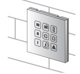
4. Install the control panel display and press it to fix.
